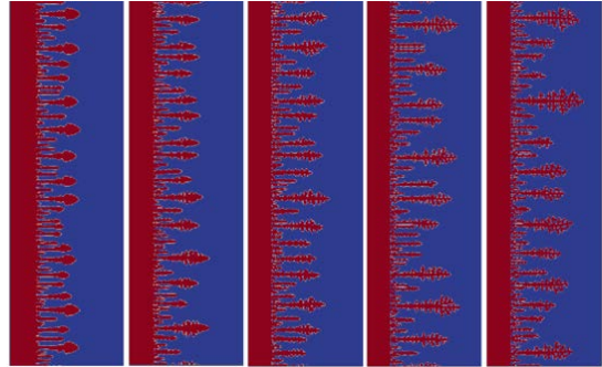
Figure 1. Current density and pulse frequencies are kept constant; figure shows the morphologies when curvature constant K=1, 2, 3, 4, 5 (from left to right); as curvature constant increases, the dendrites' mass and height and number of dendrite branches increase.
